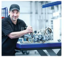
Development of operating units for valve gate nozzles to control the various pin positions hydraulically in staggered modes. For cascaded filling of injection moulded parts with several injection points, valve defects on moulded parts can be avoided this way. Messburger www.messburger.com
